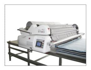
This automated machine is programmed to lay up several plies of material working quickly and efficiently, with only minor manual input i.e. people load the roles of material onto the machine, programme it and monitor the machine doing the work.
